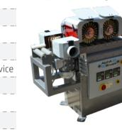
pass. All sanding brushes are reversible inverter driven for added sanding adjustment. Four 100mm (4") dust ports keep the dust contained for a clean working environment.
